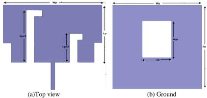
Figure 1: Geometry of proposed CPW-fed monopole antenna.
