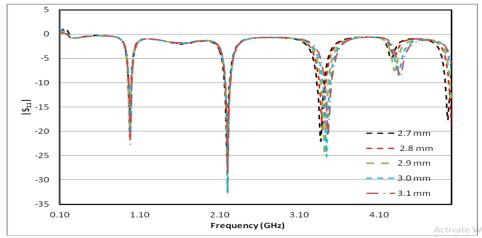
Figure 6: Return loss vs. frequency plot for variation in width of L-slot
