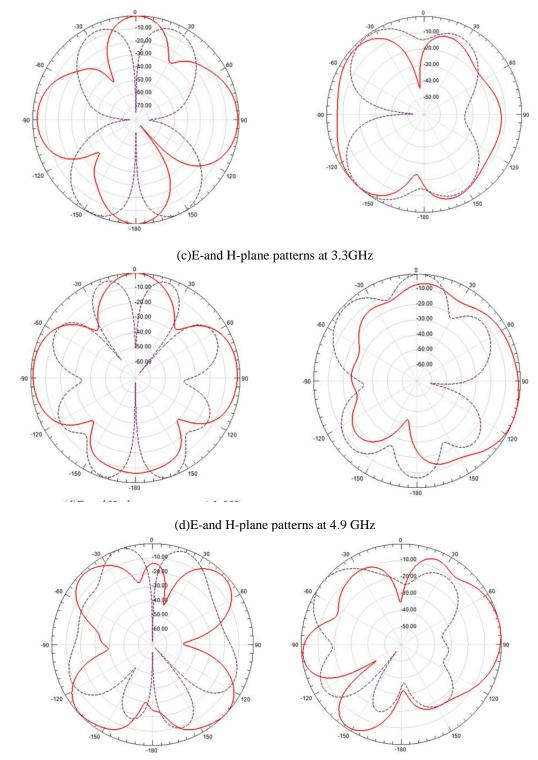
Figure 6: E-and H-plane radiation patterns at various frequencies throughout the band of operation
