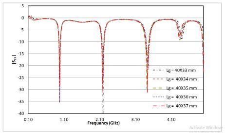
**Figure 3:** Return loss vs. frequency plot for variation in length of ground plane  $(L_{\sigma})$ .
